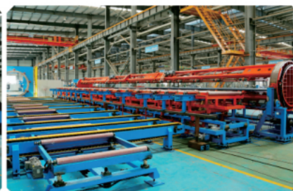
▲ 翻转码垛系统 Turnover and stacker system
